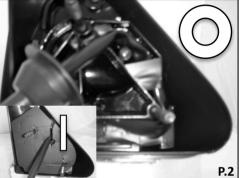
**Correct Routing**: (Photo 1) Remove foam pad and route the harness thru the pre-designated ditch up to the point where the harness enter into the door panel and STOP. (Photo 2) Duct tape can be used to avoid the harness from moving during installation. Cut foam pad along the drawn WHITE line to accommodate the harness for a perfect fit.
