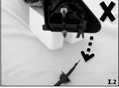
**Incorrect Routing**: (Image 1) If the harness are run over the bottom rib of the mounting base you will pinch and cut the harness when tightening the nuts. (Image 2) Pinched harness shown.
