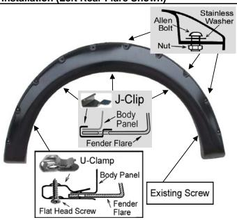
Use hex key to tight allen bolt & nut firmly on every pocket of the fender flares first, then place the flare on the vehicle with best position. Apply 3 J-Clips into the mounting slot in flare & secure it to the vehicle, 1 U-Clamp secure into the hole with flat head screw, as shown. Fasten the existing factory screw into the original location that were previously removed.
