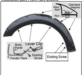
Use hex key to tight allen bolt & nut firmly on every pocket of the fender flares first, then place the flare on the vehicle with best position. Apply 3 Lever Clips secure it to the hole with existing screw, as shown. Fasten the existing factory 2 screws into the original location that were previously removed.
