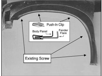
Place the flare on the vehicle with best position. Apply 2 Push-In Clip into the mounting slot in flare and secure it to the vehicle as shown. Fasten the existing factory screws into the original location that were previously removed.
