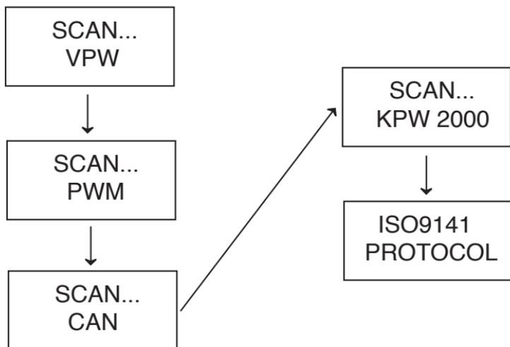
• Not all the above messages will be displayed unless protocol of the vehicle being tested is the last one—the ISO9141 protocol.
