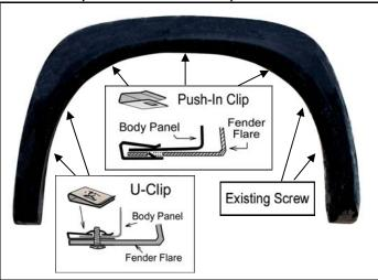
Place the flare on the vehicle with best position. Apply 3 Push-In Clip into In Clip into the mounting slot in flare and secure it to the vehicle 4 U-Clips secure into the hole with screw, as shown. Fasten the existing factory screws into the original location that were previously removed.
