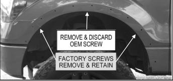
1. Remove the three existing factory screws with proper wrench and save two screws for reinstallation as shown.
