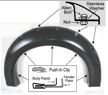
Use Torx Bit to tight allen bolt & nut firmly on every pocket of fender flare, then place the flare on the vehicle with best position Apply 5 Push-In Clip into the mounting slot in flare and secure it to the vehicle, as shown.
