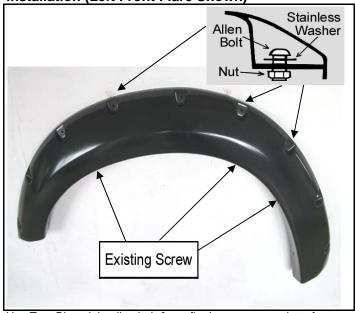
Use Torx Bit to tight allen bolt & nut firmly on every pocket of fender flare, then place the flare on the vehicle with best position. Fasten the existing factory screws into the original location that were previously removed.
