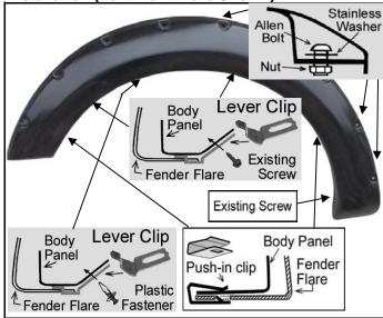
Use Torx Bit to tight allen bolt & nut firmly on every pocket of the fender flare, then place the flare on the vehicle with best position. Apply 3 Lever Clips secure it to the hole with 2 existing screws and 1 expanding fastener. Apply 2 Push-In Clip into the mounting slot in flare and secure it to the vehicle. Fasten the existing factory screw into the original location that were previously removed.
