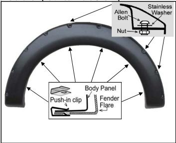
Use Torx Bit to tight allen bolt & nut firmly on every pocket of the fender flare, then place the flare on the vehicle with best position. Apply 6 Push-In Clip into the mounting slot in flare and secure it to the vehicle, as shown.
