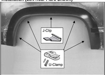
Place the flare on the vehicle with best position. Apply 1 J-Clips into the mounting slot in flare and secure it to the vehicle, 4 U-Clamps secure into the hole with hex screw, as shown.
