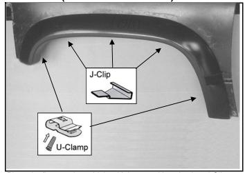
Place the flare on the vehicle with best position. Apply 3 J-Clips into the mounting slot in flare and secure it to the vehicle, 2 U-Clamps secure into the hole with hex screw, as shown.
